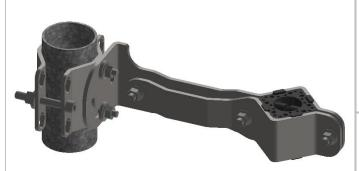
On a vertical, horizontal (or oblique) **cylindrical mast** with an outer diameter of **40 mm**, use the provided V brackets without the reduction shims.
