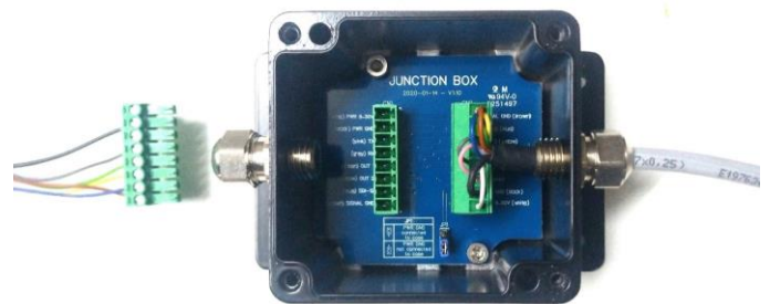
Sensor cable (left) and Junction box
