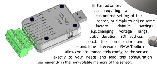
■ Free download the ISAW-Toolbox software suite at www.isaw-products.com. Connect the sensor to your computer using the USB dongle accessory. The USB dongle has an 8-pin quick connector for the sensor's wires, a built-in power converter, and a USB plug for direct connection to a Windows, Linux, or Mac OS machine.
