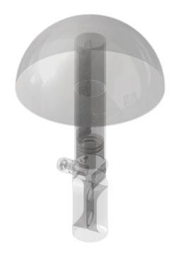
the impact transferred to the sensing surface (the higher the transfer of momentum to the sensing surface, the higher the impulse acoustic response caught by the microphone). For each individual impact, the momentum that is transferred to the sensing surface depends on the particle's mass, velocity, type and incidence angle on the hemisphere, so all these factors have to be taken into account when determining the size classes, type, amount and intensity of the precipitation.
