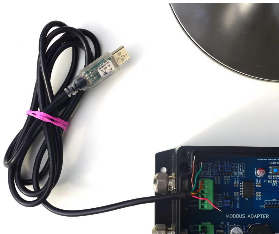
Picture 6: RS485/422 adapter connected to the MODBUS connector of the Modbus adapter
