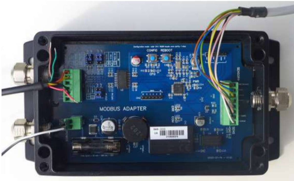
Picture 2: Modbus adapter connectors. Left: MODBUS and POWER connectors. Right: INSTRUMENT connector.
