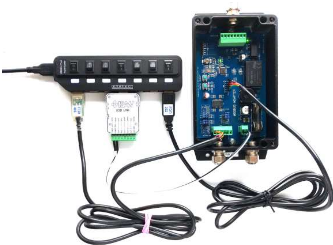
Hardware setup with USB hub and Modbus adapter
