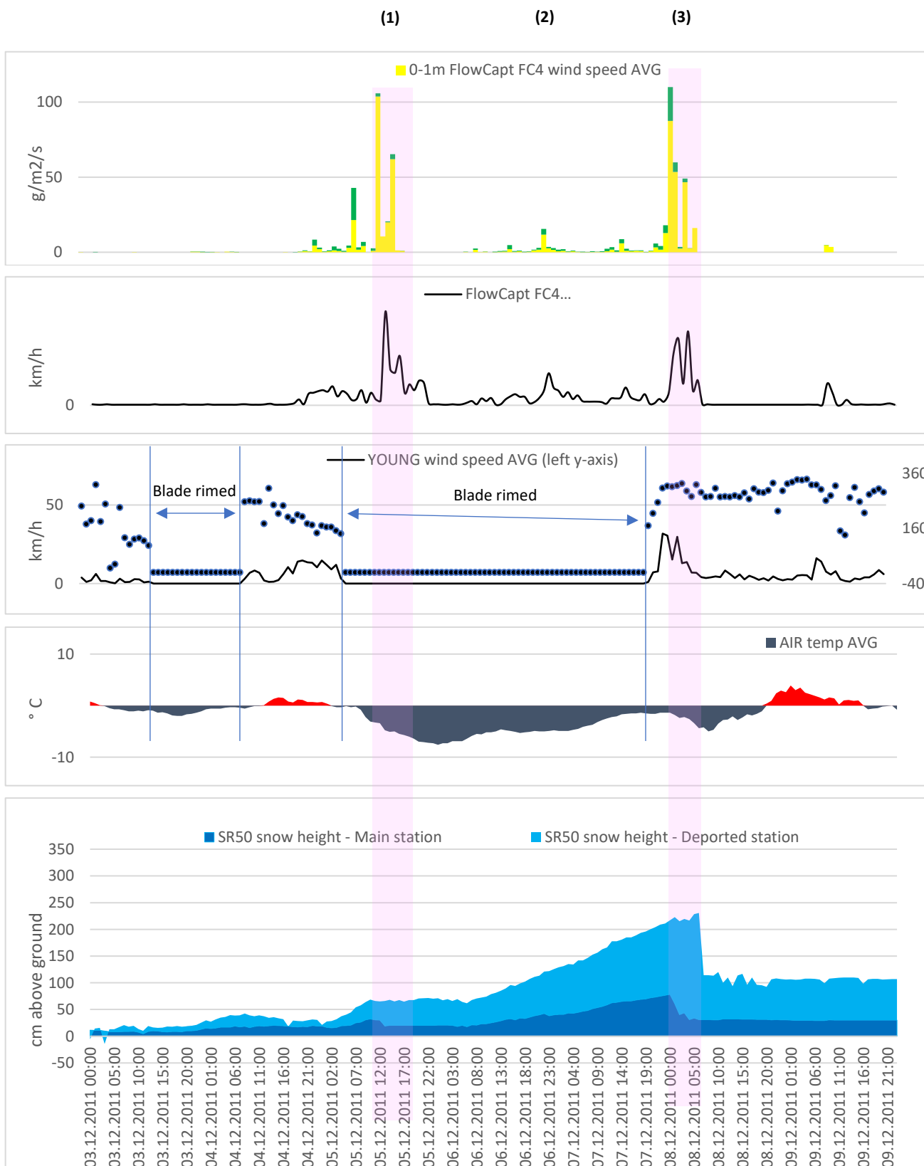
Measurements from 3 to 9 December 2011, at the station in Celliers (Savoie, France). In period 1, we can see a first episode of wind transport: the FlowCapt instruments record transport, the anemometer, frosted, does not give any indication, the main snow depth decreases while the other increases. On period 2: we see a snowfall without much transport: The FlowCapt instruments don't register much, the snow depths both increases. On Period 3: we see a well-marked transport episode, with strong erosion, the anemometer has finally unlocked. The effectiveness of the artificial release that followed this period is clearly visible.
